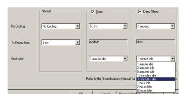
In Deep Sleep mode, the receiver cycling time can be as slow as one second. The TB8100 switches off the PMU DC-DC converter and runs using the standby power supply module. Because the highly efficient standby supply provides 10W and only powers the reciter, power savings are dramatic.
