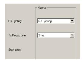
Receiver cycling can provide additional power saving by turning the receiver off and then on again for a brief period to check if there is a signal. Receiver cycling time is selectable with 0, 5, 10, or 20 mS options.
